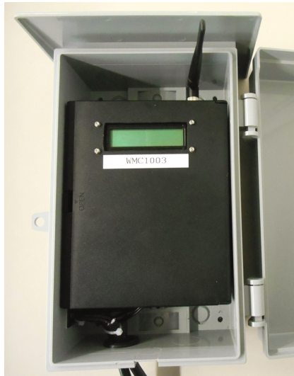
Fig. 5. Solar power monitoring system, “SunMieru”
