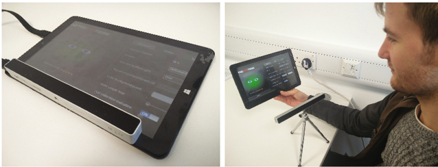
Fig. 5. A demonstration of the compact nature of the portable eye movement lab system.
