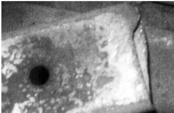
Fig. 7. Part of leaf spring after breaking
