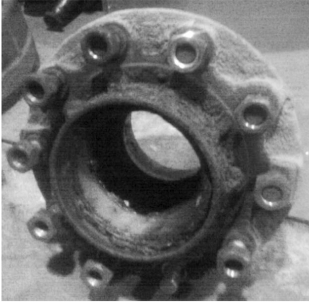
Fig. 8. Wheel part of Yutong 6108 bus with studs
