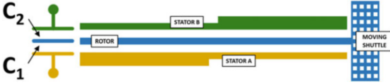
Fig. 3.1 Sketch of a typical differential capacitive sensing cell for a MEMS structure. Stators A and B are anchored to chip substrate and they form a differential capacitor with rotor
