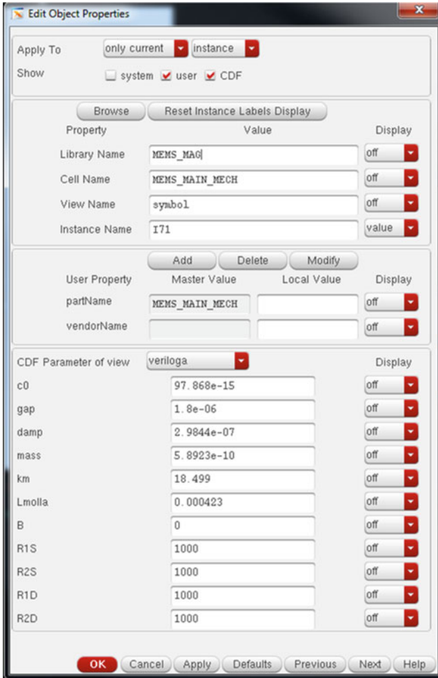
Fig. 9.8 The MEMS device can be added in the Cadence ® —Virtuoso simulation tool as a basic building block of the circuit and its mechanical parameters can be set in object properties window
