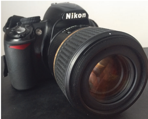
Fig. 2.3 My current camera, Nikon D3100 with a 60 mm F/2 Tamron macro lens. A number of cameras are useful. Woodrow Wilson of www.clinicalimaging.com.au recommends consumer grade DSLR with lens between 60 and 100 mm
