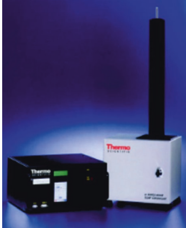
Fig. 6 Particulate sampler monitor installed by the New York State Department of Environmental Conservation
