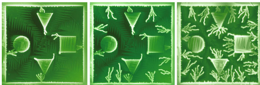
Fig. 5.24 MOI of magnetic field distribution in a Nb film with holes of different geometries. From left to right , the applied field is 2.25, 3.15, and 4.20 mT (from [56])
