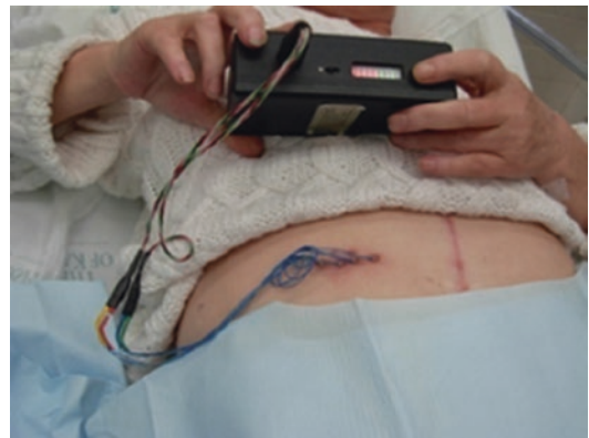
Fig. 25.1 Two-channel gastric pacing prototype device pulse generator ( black box ) is attached to external wires in a patient with refractory GP. These external wires stimulate electrodes that were surgically attached to the serosa of the stomach when the device is activated after meals
