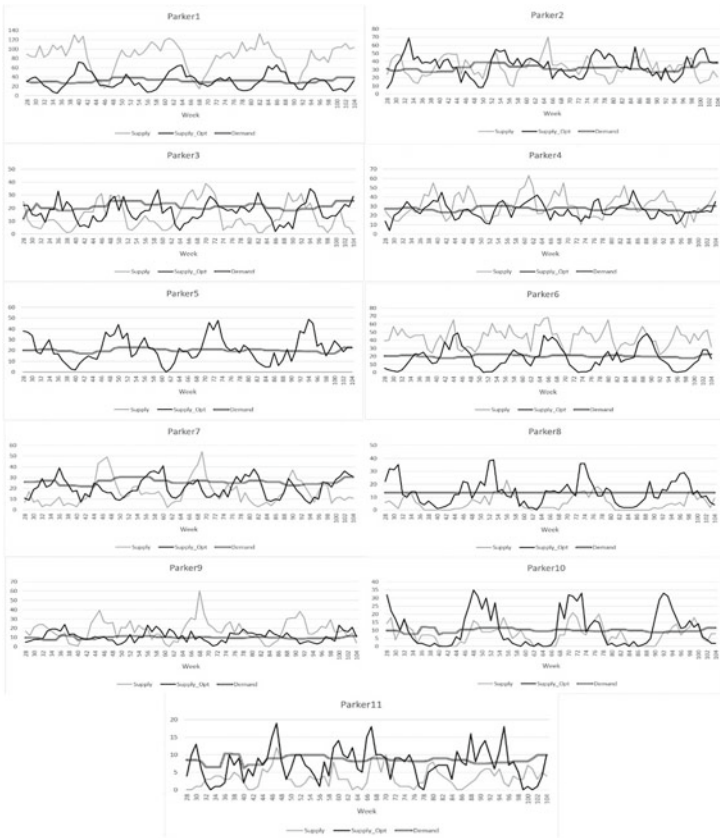
Fig. 7. The line graphs between the supply and demand of the 11 packaging plants in the original and the optimized model during 28-104th weeks
