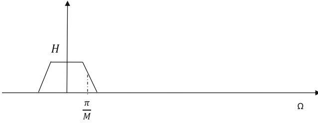
Fig. 3 Frequency response of prototype filter
