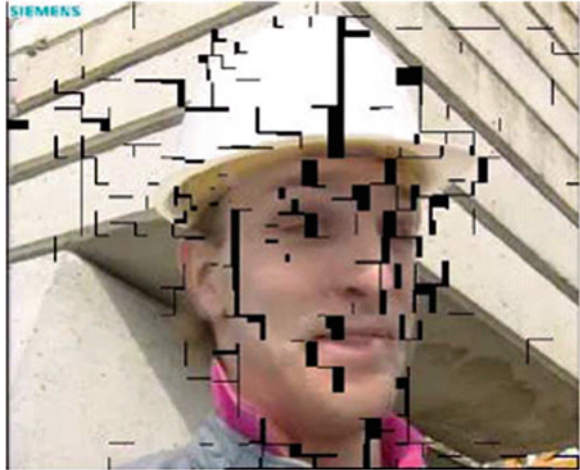
Fig. 17 The problems on overlaps and holes. The black regions are not pointed by reference pixels, which generate the holes
