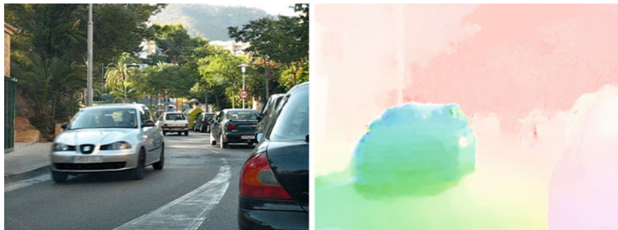
Fig. 11 An example of MVF estimated by optical flow estimation [23]. The MVF includes MVs of each pixel. The color coding of the MVF is explained in the evaluation method section
