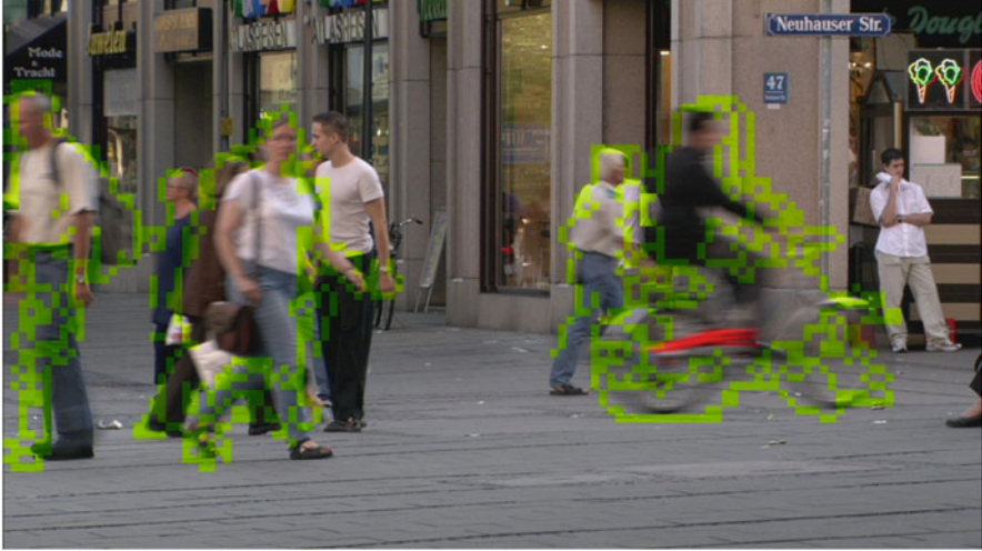
Fig. 21 An example of possible regions with visual artifacts detected by [30]. These regions mostly reside near the boundaries of moving objects
