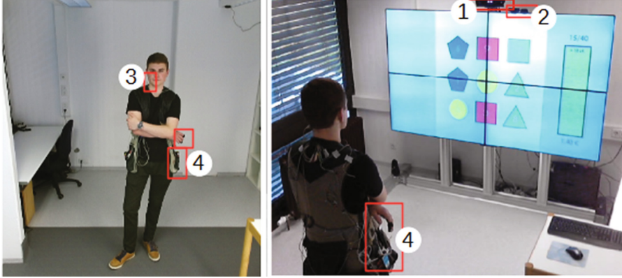
Fig. 2. Overview of the setting with sensors: (1) MS Kinect v2, (2) frontal webcam, (3) wireless headset, (4) GTec g.MOBilab+ physiologic sensor with sensors attached to the users body.
