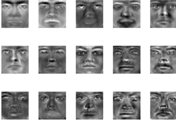
Fig. 7. Group of 15 TensorFaces basic vector from HSVD tensor decomposition using YALE dataset
