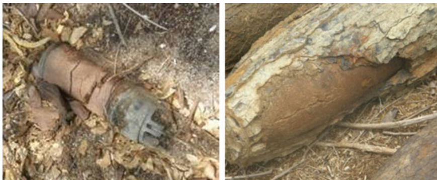
Fig. 5 Explosive fill exposed by corrosion of unexploded ordnance (UXO) casings [65]
