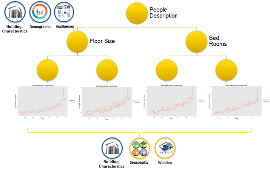
Fig. 2. The hybrid model design. Ctree model is used based on time-independent predictors for grouping the buildings into several homogeneous groups. Afterwards, an individual linear regression model is fitted for each group based on building characteristics and time-dependent factors.
