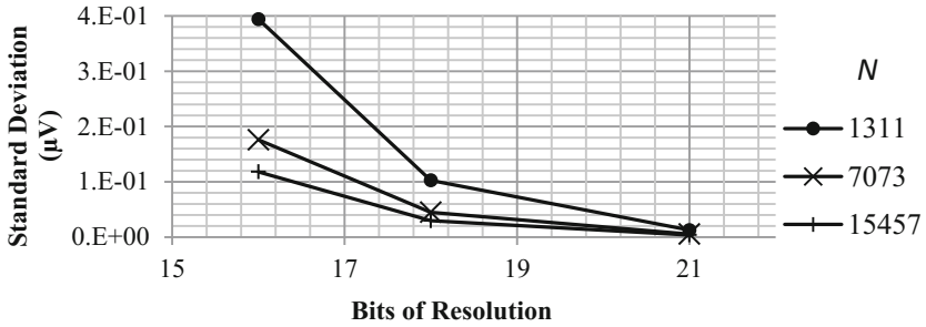
Fig. 4. Standard deviation of fundamental frequency amplitude deviations to nominal values ( \mu\text{V} ) obtained for N_{bits} and N values - only quantization considered
