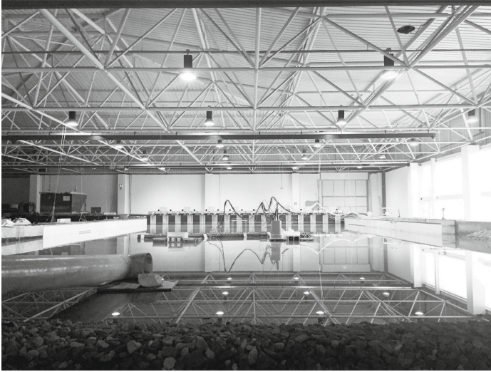
Fig. 1. Hydrodynamic experimentation wave basin with the scaled port model. Wave-maker in the background
