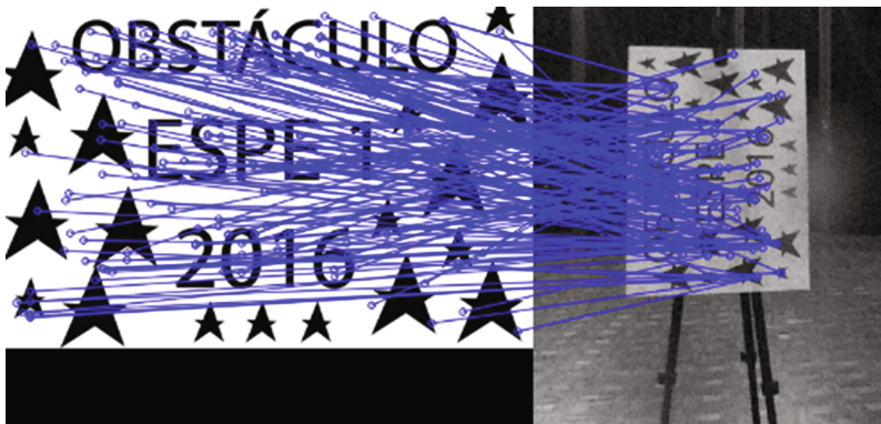
Fig. 1. Matching between image from database and real-time image at UAV
