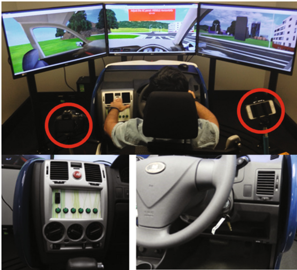
Fig. 1. Driving simulator (Forum 8) setup, camera views for recording middle/driver side gestures.
