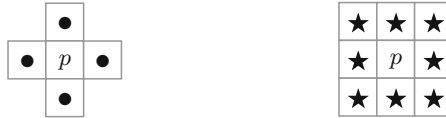
Fig. 1. The considered adjacency relations on the square grid. Set N_4(p) contains point p and the four points marked “•” (left), and set N_8(p) is formed by p and the eight points marked “★” (right).
