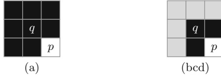
Fig. 8. Configurations associated with Theorem 2 when (the originally black) simple point p is matched by the template in Fig. 3a and q = q_1 .
