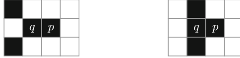
Fig. 12. Configurations associated with Proposition 4. Point q is a non-simple and border point, and p is a line end point in (8, 4) pictures (left) and (4, 8) pictures (right). We can state that q remains non-simple after the deletion of p . Hence line end point p is not a simplifier.
