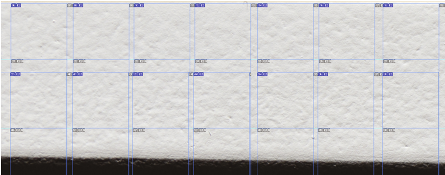
Fig. 1. Example of images of the surface of furniture elements. Small images of size 300 \times 300 like those outlined with blue lines and marked with small dark blue icons were cut for the training and testing processes. Each of these images contained only the evenly illuminated surface of the object. (Color figure online)
