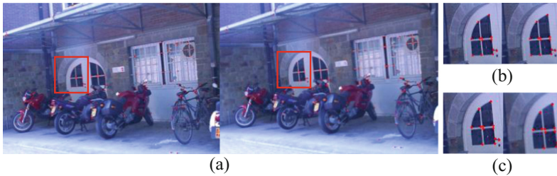
Fig. 4. Feature points detected for two bike images and correspondences of them. (a) Feature points detected in bikes1 (left) and bikes2 (right). (b) Enlarged sub-images in red frames of (a). (c) Correspondences of feature points computed using homography matrix. (Color figure online)
