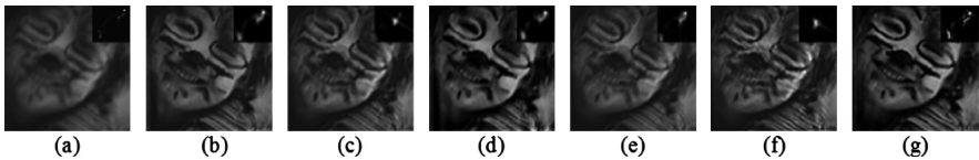
Fig. 5. Deblurring results on synthetic image. (a) Blurred image and the ground truth blur kernel. (b)–(f) are the deblurring results of Refs. [10], [6], [11], [16], [13], respectively. (j) is our deblurring results.
