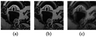
Fig. 1. Images are contaminated by blur kernels in different size. (a) clear image. (b) blur kernel size is 5 \times 5 . (c) blur kernel size is 27 \times 27 .
