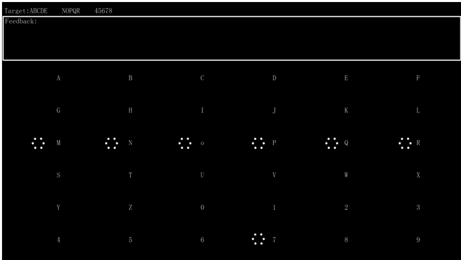
Fig. 1. Screenshot of the visual stimuli. The top characters are the targets in the offline experiments. The ‘Feedback’ region is used to demonstrate the results in the online experiments. This picture shows one moment during the stimuli presenting.
