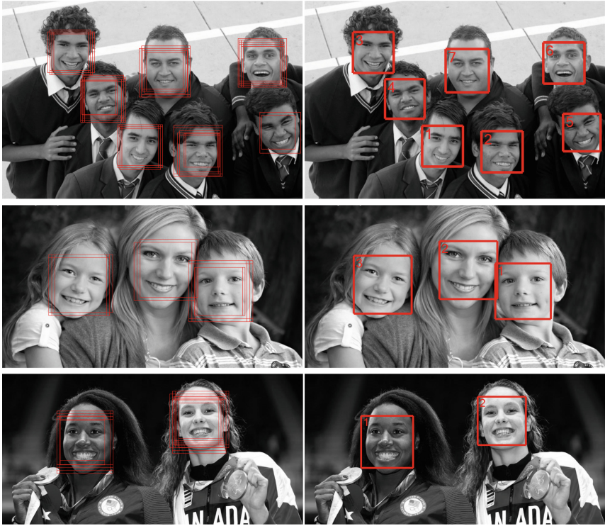
Fig. 4. Examples of single outcomes returned by the Fourier-based detector: before grouping positive windows (left-hand side) and afterwards (right-hand side).
