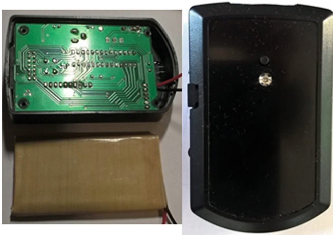
Fig. 4. The developed device embedded inside the plastic casing with dimensions: 90 \times 58 \times 18 mm.
