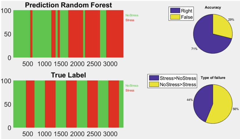
Fig. 7. Result of a classification of a stress test: predictions of the random forest (upper left), true labels of the stress test (bottom left), classification accuracy (upper right), and type of errors (bottom right).
