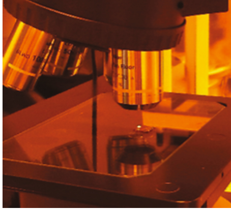
Fig. 5. The microscope used to explore the fabrication defects of the organic solar cells.
