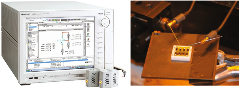
Fig. 3. Agilent B1500A semiconductor device analyzer (Keysight Technologies) (left), measurement probe station (right).
