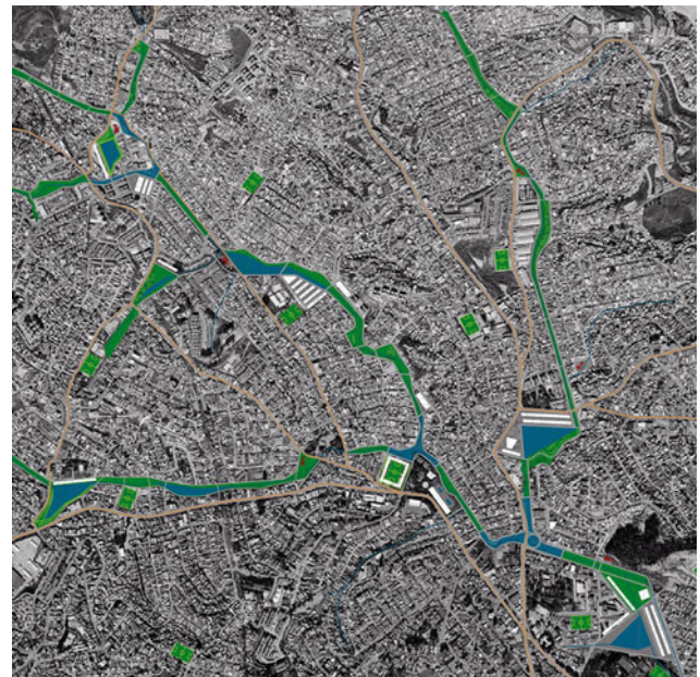
Fig. 28.6 MMBB Arquitetos São Paulo, Watery Voids, 2008. Green/Blue structure for managing rainwater in Sao Paulo
