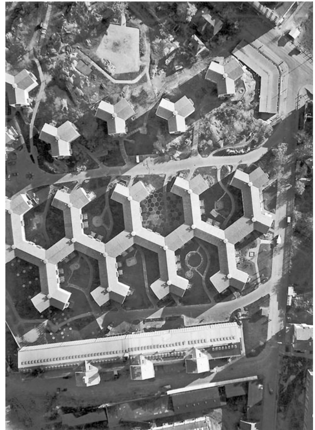
Fig. 6.4 Sven Backström & Leif Reinius, residential development, Gröndal, Sweden, 1944–46. Aerial view of the suburb where the strong geometric design of the star-shaped dwellings can be observed, either forming small, interlocked 3/4-storey blocks creating hexagonal courtyards between them, or freely placed seeking the best orientation
