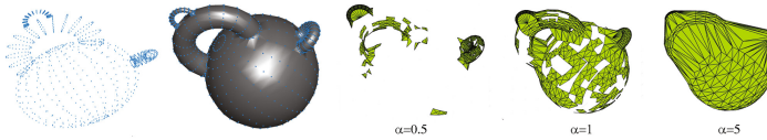
Fig. 1. From left to right: a point set, a triangulation and a sequence of three alpha shapes with increasing values of \alpha .
