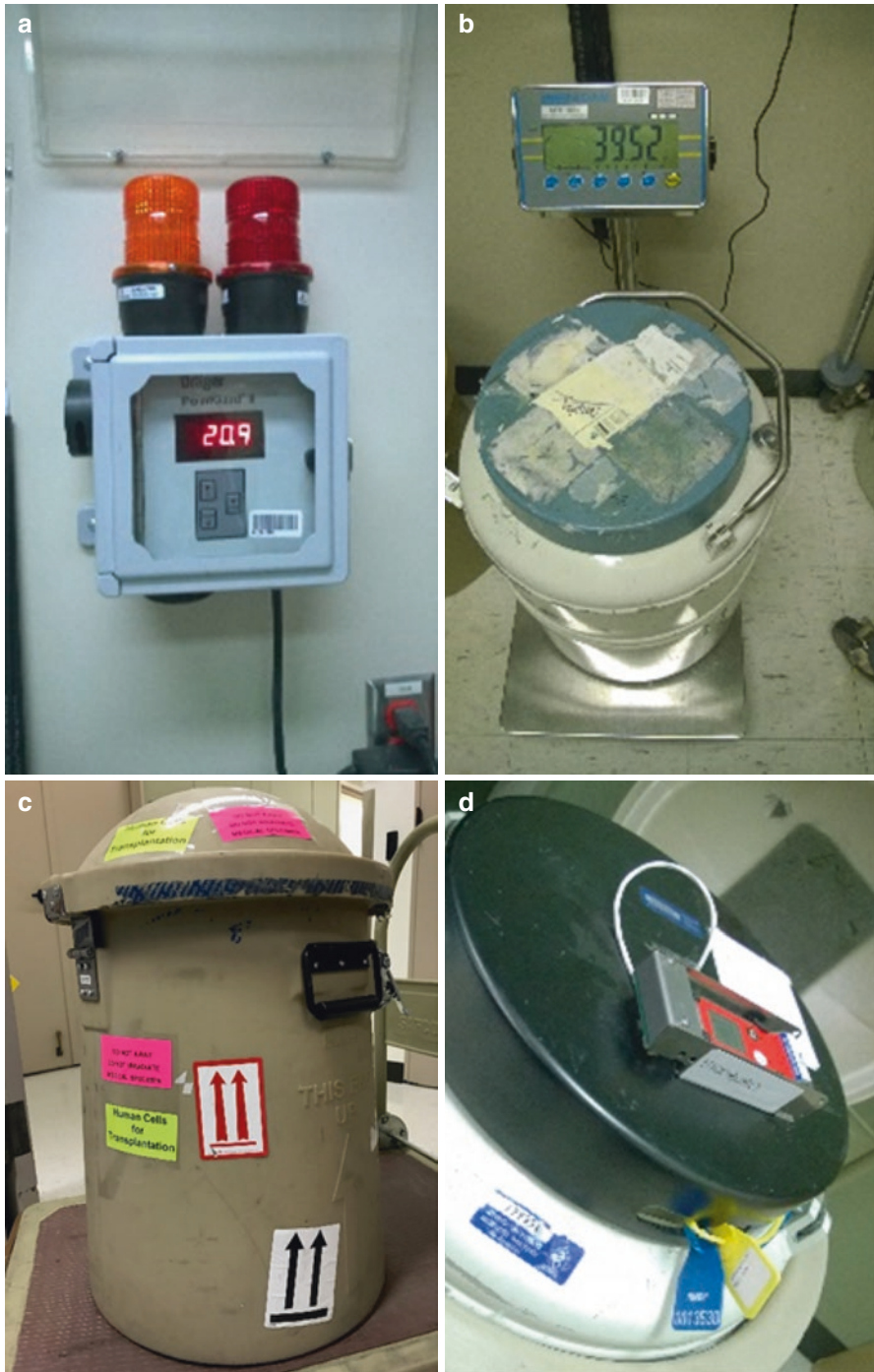
Fig. 12.4 (a) Oxygen level sensor, (b) charged dry shipper weight, (c) packaging and labeling, and (d) tamper proofing the dry shipper
