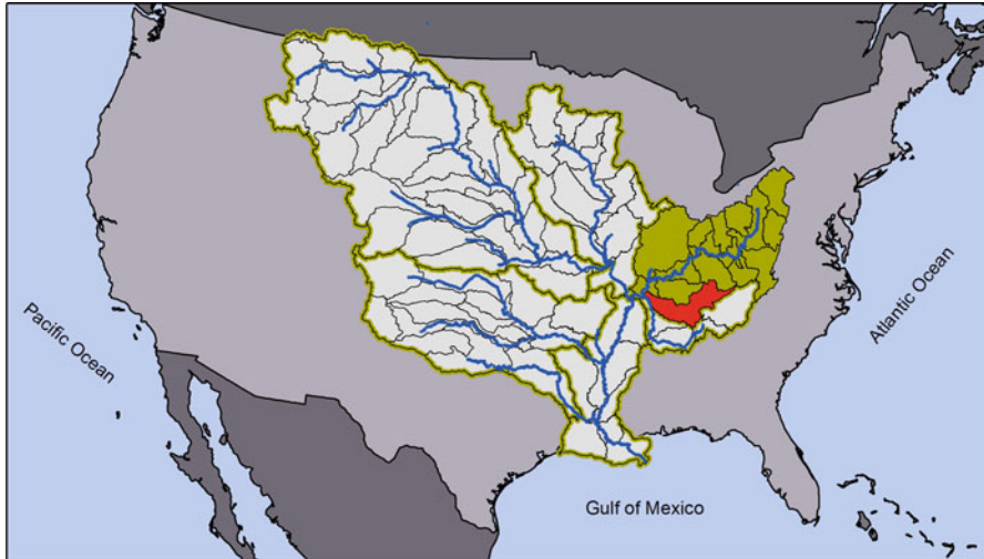
Fig. 1 Division of the complete Mississippi River Basin into six HUC2 regions and 84 HUC4 sub-regions. HUC2 region 05 and HUC4 region 0531 are highlighted in solid colors
