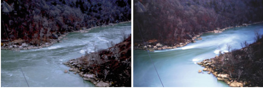
Fig. 1 Two images of the same Niagara Falls downstream flow. The left image is an exposure of 0.4 s, while the right-hand image is exposed for 50 s. Note the flow features visible in the right-hand image (streamlines, bow waves, standing waves, vortices, etc.) that are not clearly visible or invisible in the left image
