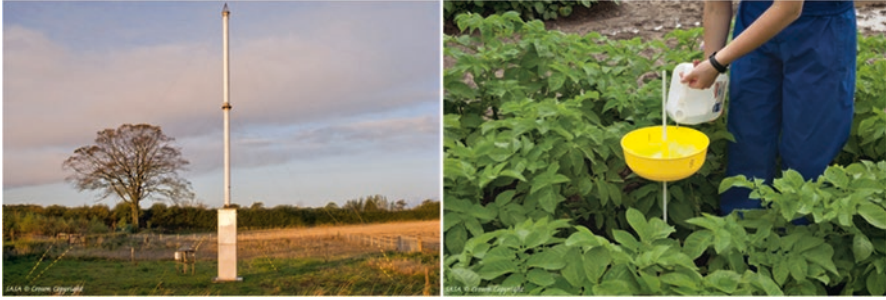
Fig. 6.7 Suction trap (Rothamsted-type 12.2 m high) ( right panel ) and water pan trap ( right panel ) currently used for aphid monitoring (Courtesy of SASA, Crown copyright)
