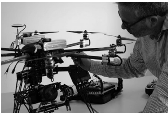
Fig. 5 Eight-rotor drone. Completing the list of verification prior to transport to the place of flying
