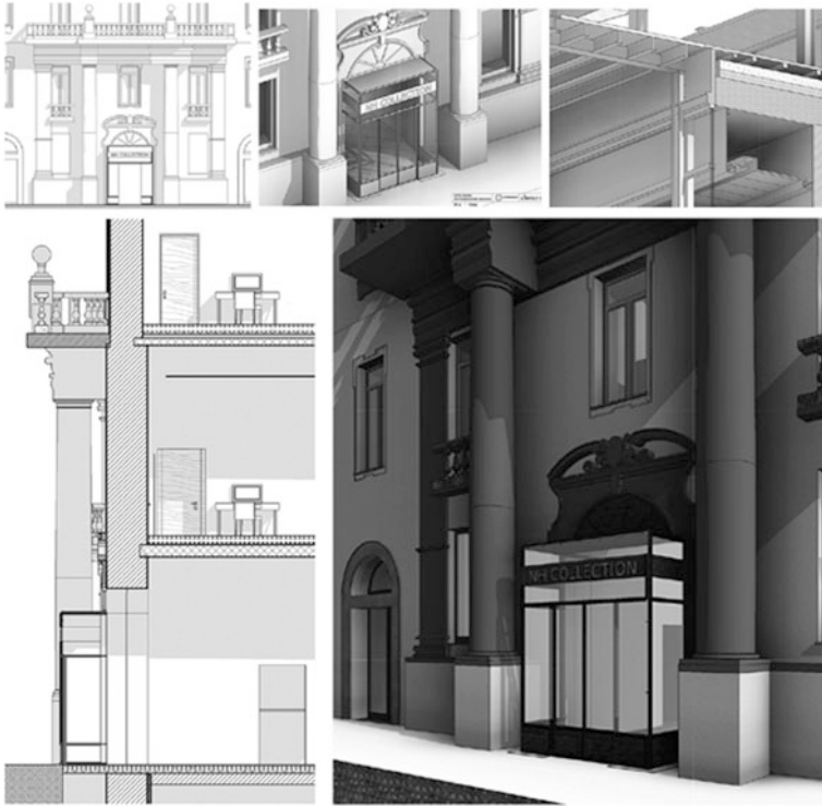
Fig. 7 Section, elevations and conceptual views, construction details and render of the main entrance to the new Carlina hotel, in Turin. The digital model is simultaneously used to operate functional, stylistic and material/color choices. Image courtesy architect. F. De Giuli (2015)
