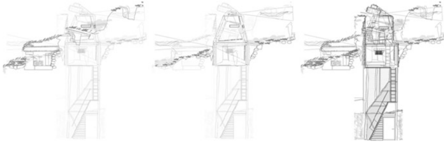
Fig. 2 Overlays successive sections of the three cases, highlighting in the first one the trenches, in the second one the camera obscura and the third one the total overlay
