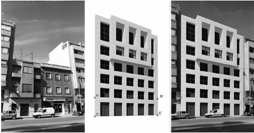
Fig. 6 Homographic transformation of the environment snapshot “stretching” the environment image until the points A, B, C and D match their counterparts A', B', C', D'
