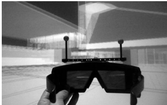
Fig. 7 The goggles have devices that can identify the observer’s position and orientation, updating the images projected on the screens in real time
