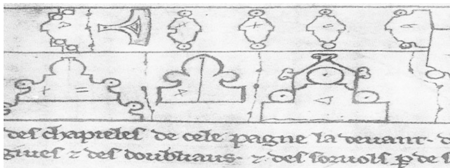
Fig. 1 Folio 32 detail of Villard de Honnecourt's Album , with drawings of details of the stones cutting pattern for Reims's Cathedral. In the image, according to the caption: "Here are the templates of this page chapels, those of the vain ones and windows, of the ogives, of the transverse ribs, and above, the formers." (Villar de Honnecourt. [13th Century] 1991, plate 63, p. 138 translation)
