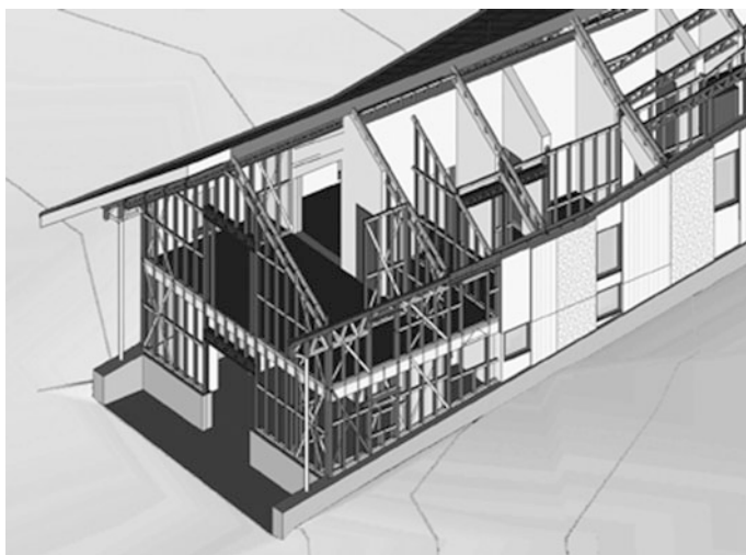
Fig. 10 Isometric cutaway view of structure and finishing. Author Lewis Dal Magro
