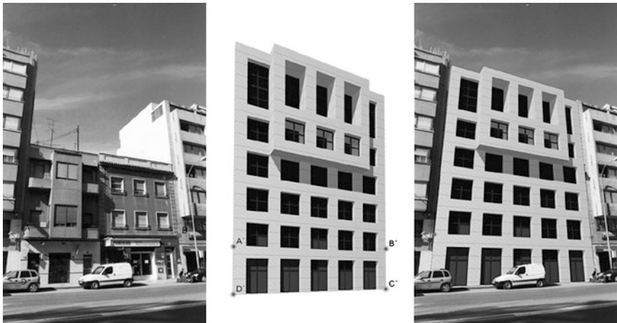
Fig. 7 Homographic transformation of a photo—perspective “stretching” the points A, B, C and D and matching them with their counterparts A', B', C', and D'
