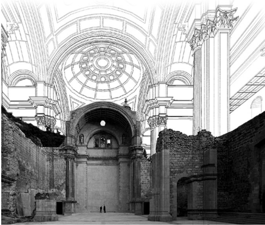
Fig. 7 Overlay of interior spaces rebuilt on the ruins of Saint Mary of Cazorla church. Jesús Estepa Rubio drawing
