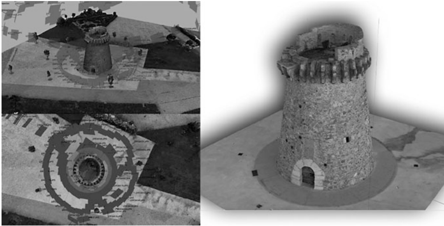
Fig. 3 Photomodeling process by SfM and digital 3D modelling
