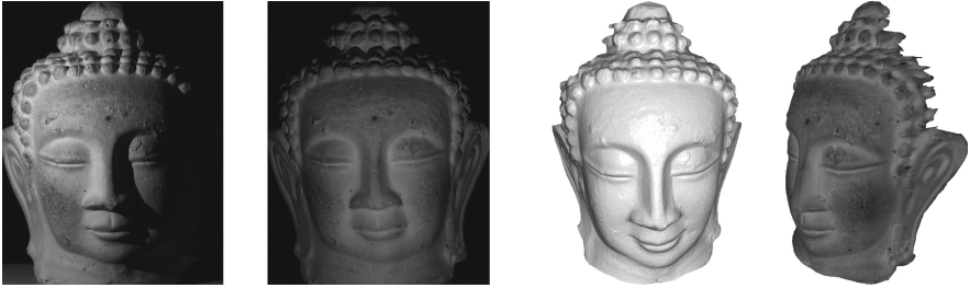
Fig. 1. Left: 2 out of m = 8 images of a plaster statuette. Each image is acquired while turning on one different nearby LED with calibrated position and orientation, but uncalibrated intensity. Right: result of our semi-calibrated PS approach, which automatically estimates the shape, the reflectance (mapped on the 3D-reconstruction on the rightest figure) and the intensities.
