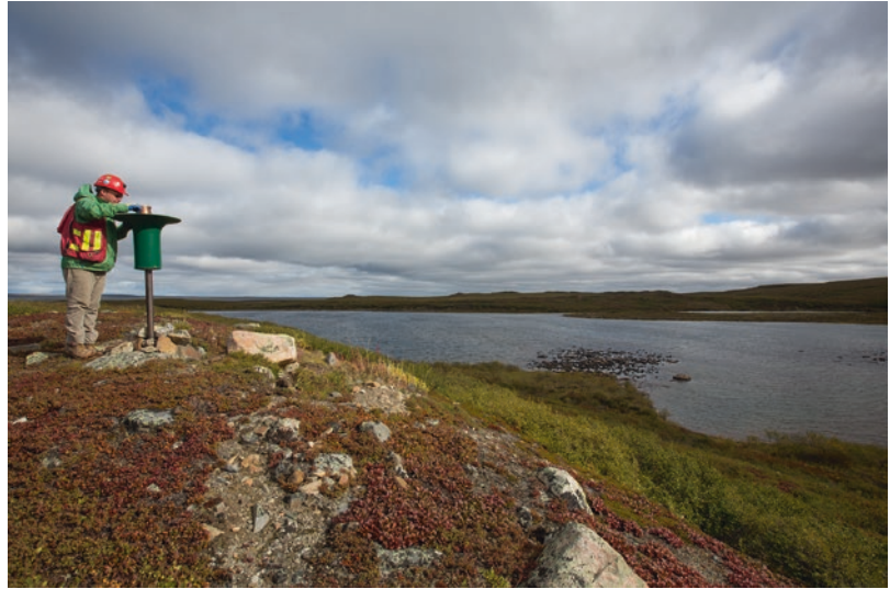
■ Fig. 7.22 Air quality monitoring at a dust collection point near the mine (Image courtesy of Rio Tinto)
