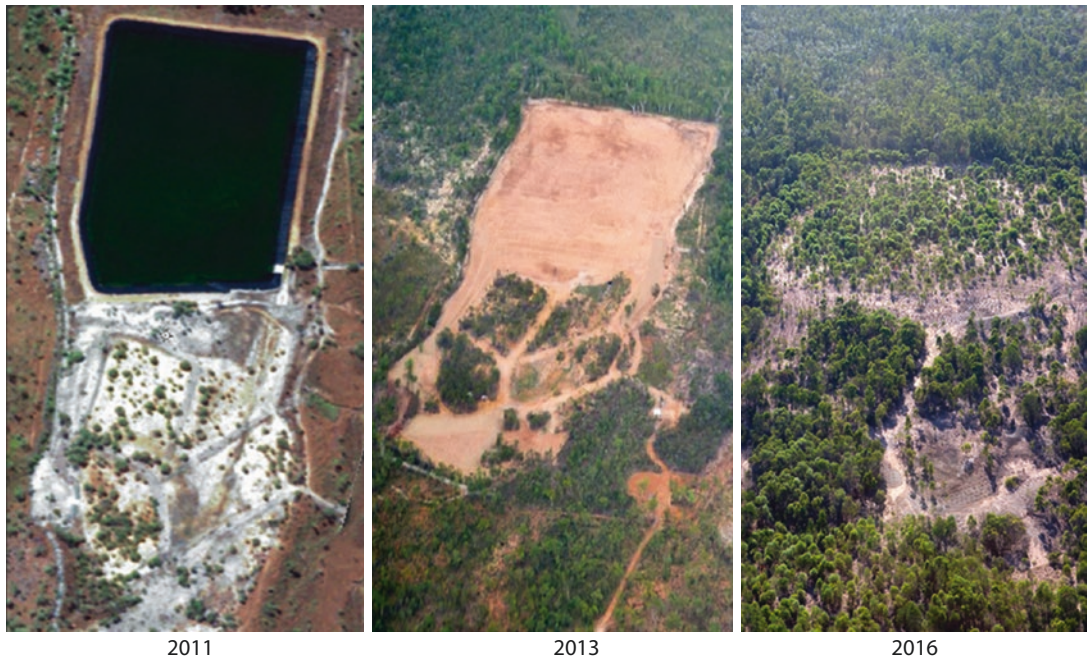
■ Fig. 7.38 Evolution of Water Management Pond rehabilitation from 2011 to 2016
