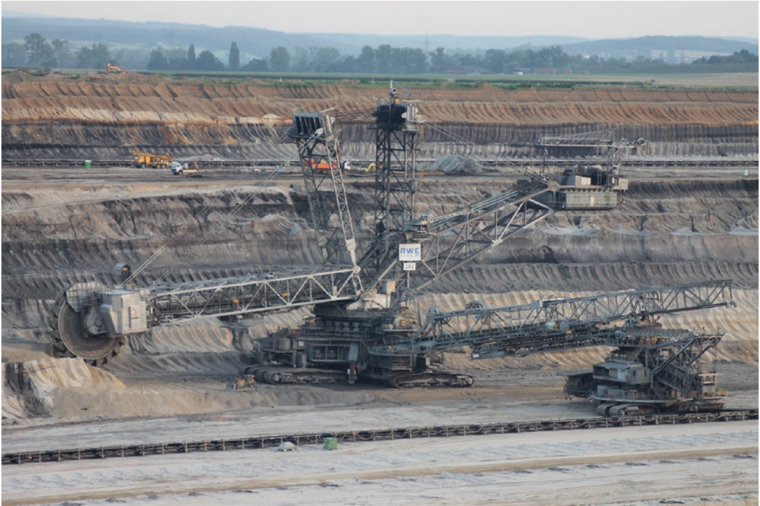
■ Fig. 5.14 Bucket wheel excavator (Image courtesy of ThyssenKrupp)
