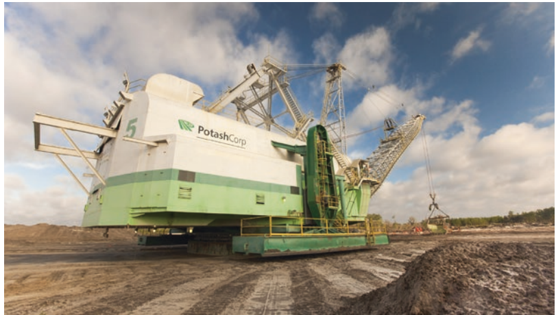
■ Fig. 5.17 Dragline operating in a phosphate mine (USA) (Image courtesy of PotashCorp)
