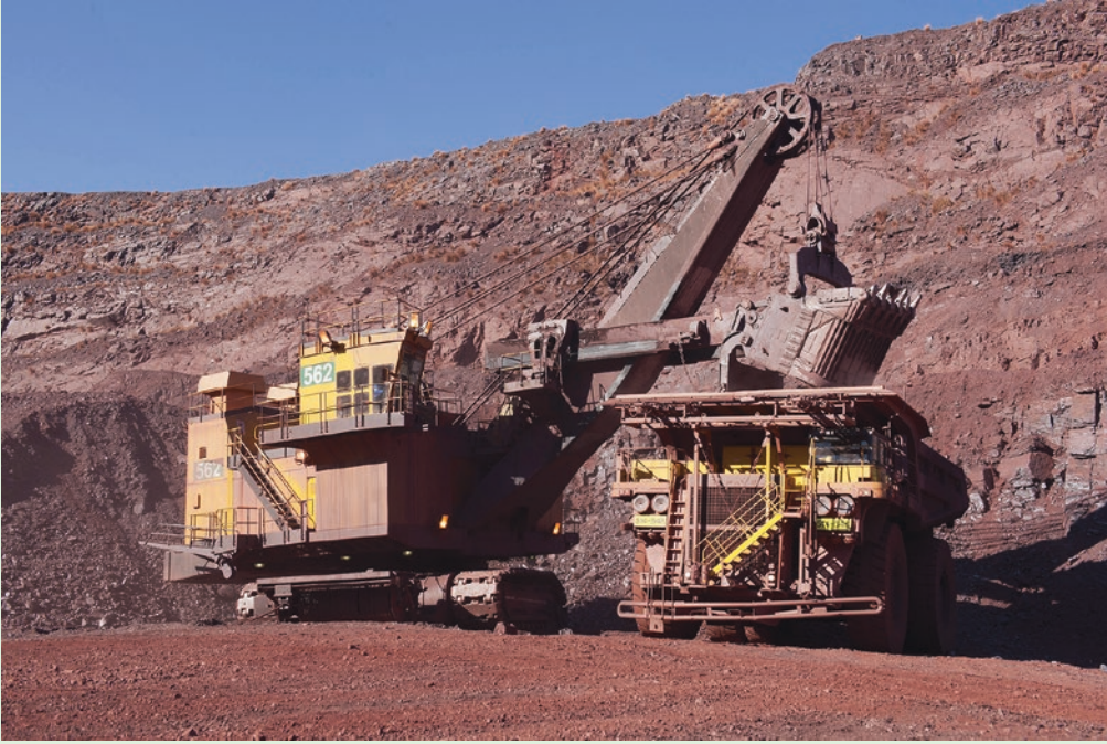
■ Fig. 5.12 Optimal combination of a large shovel and truck (Image courtesy of Anglo American plc)
