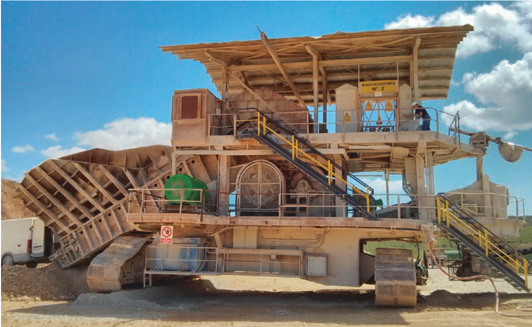
■ Fig. 5.20 In-pit crushing (Image courtesy of Octavio de Lera)
