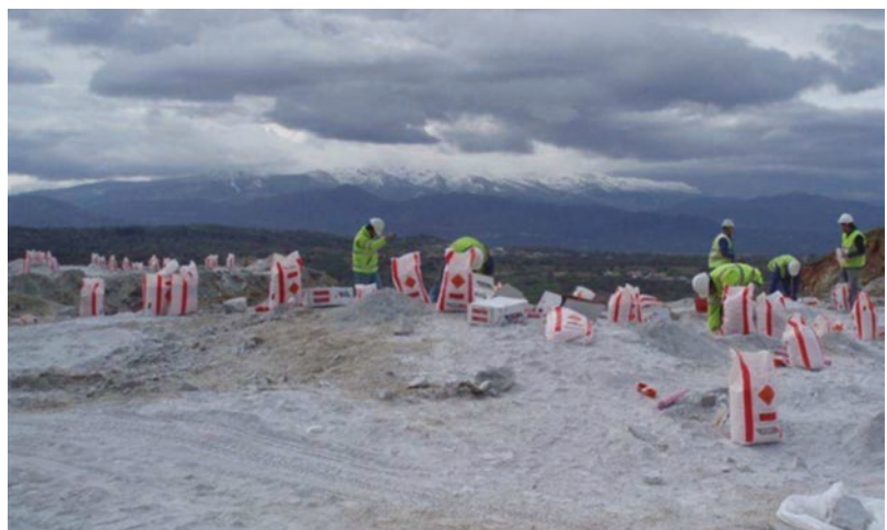
■ Fig. 5.94 Grade control prior blasting (Spain) (Image courtesy of Daytal Resources Spain, S.L.)
