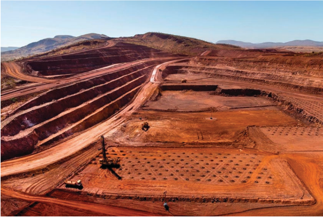
■ Fig. 5.8 Appropriate drilling and blasting procedures are fundamental to develop the final walls of the open-pit (Image courtesy of Rio Tinto)
