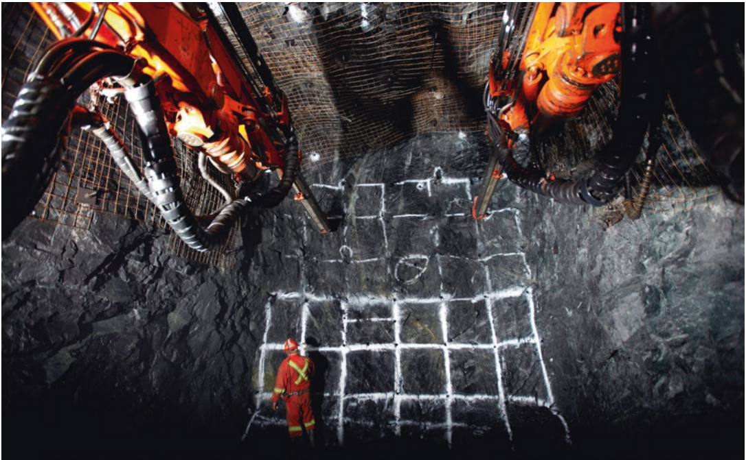
■ Fig. 5.92 Driller marking rock face (Image courtesy of North American Palladium Ltd.)
