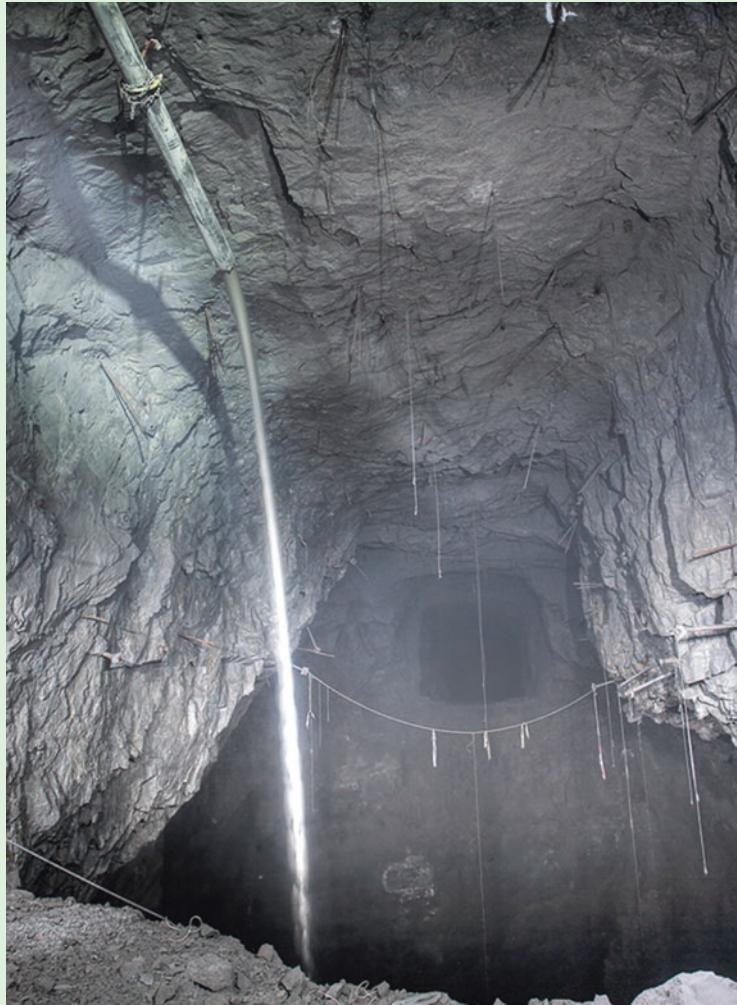
■ Fig. 5.63 Paste fill used in the stope (Illustration courtesy of Matsa, a Mubadala and Trafigura Company)
