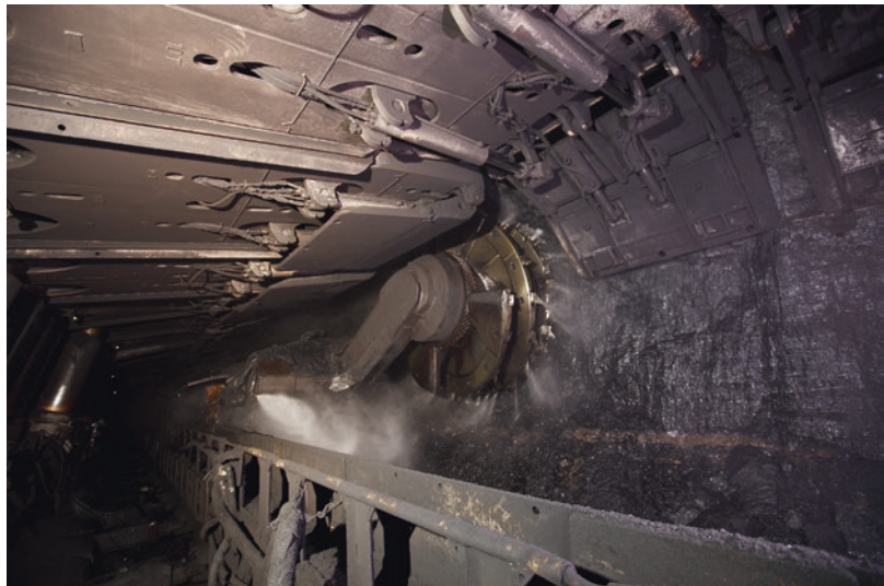
■ Fig. 5.68 Coal seam mined by longwall method using continuous miner (Image courtesy of Anglo American plc)
