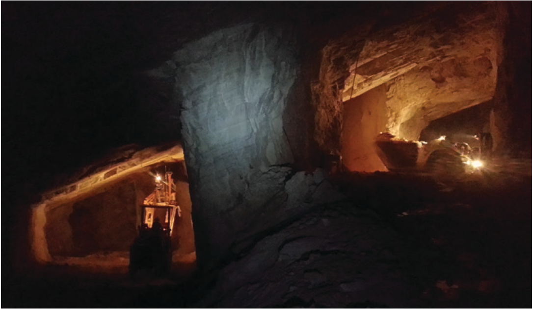
■ Fig. 5.59 Two rooms and one pillar in a room-and-pillar underground system (Spain) (Image courtesy of Pedro Rodríguez)
