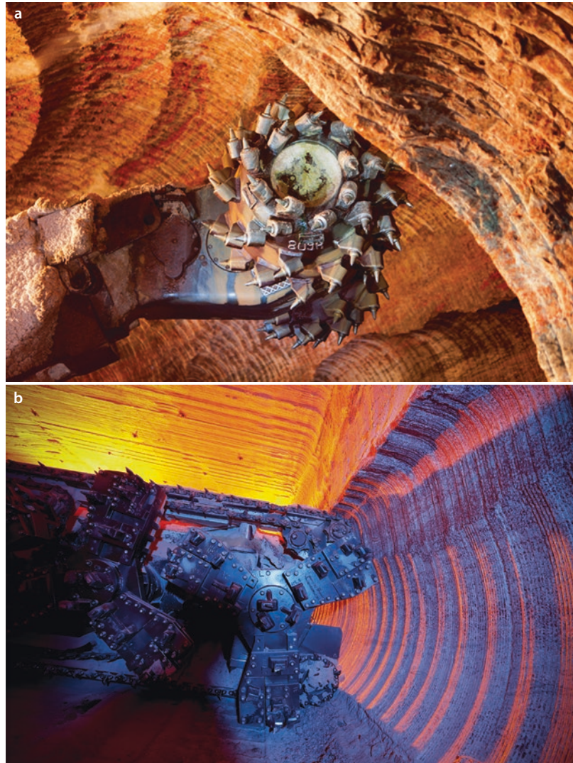
■ Fig. 5.53 Different types of continuous miner (a image courtesy of Iberpotash; b image courtesy of PotashCorp)
