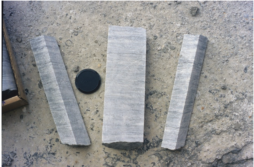
■ Fig. 4.14 Half and quarter core as samples (Image courtesy of Pedro Rodríguez)
