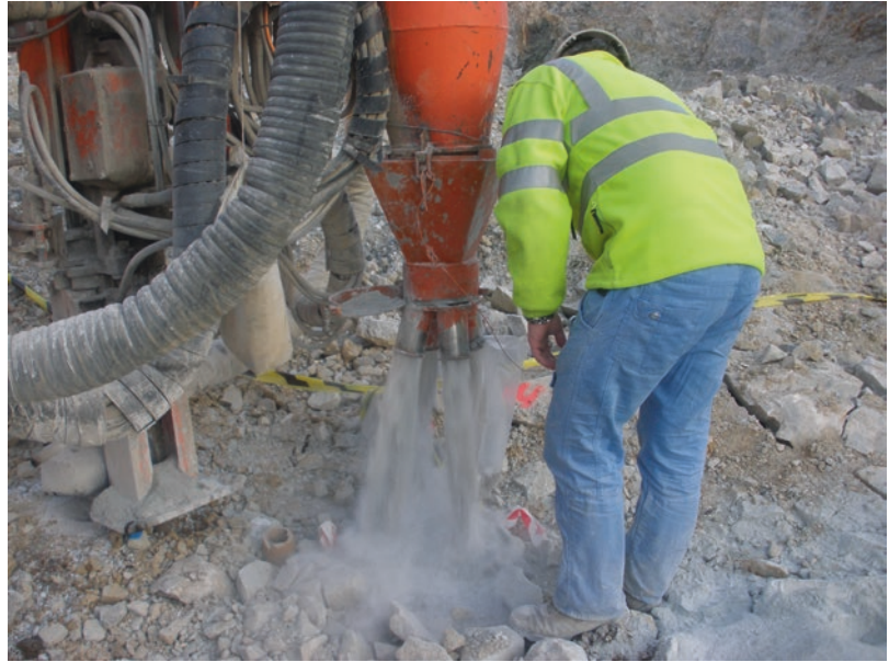
■ Fig. 4.2 Taking samples for grade control (Image courtesy of Alicia Bermejo)
