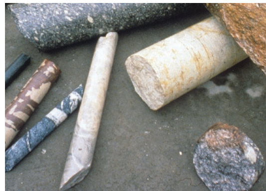
■ Fig. 4.41 The volume, size, and position in space of a sample is the «support»
