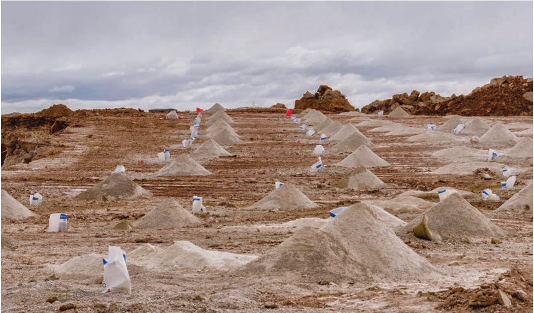
Fig. 4.5 Sampling grid in blasting
