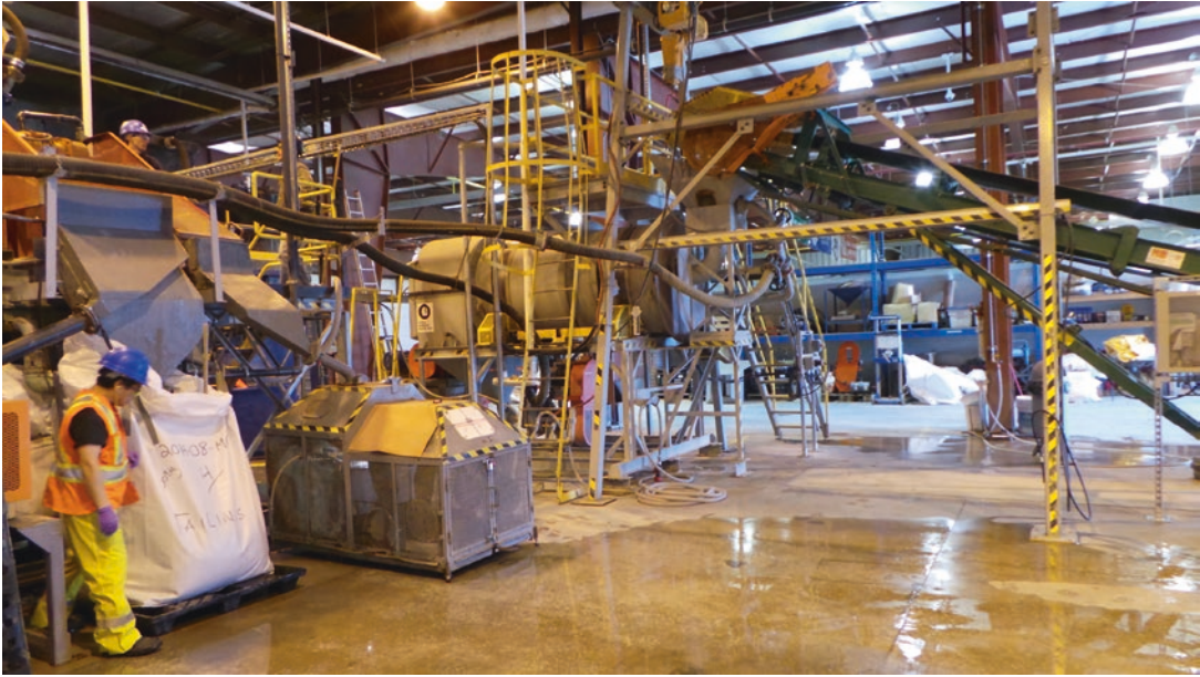
■ Fig. 4.10 Bulk sample plant where kimberlite samples are being treated (Image courtesy of De Beers)
