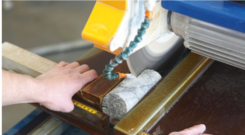
■ Fig. 4.15 Core cutting with a diamond saw (Image courtesy of Euromax Resources)
