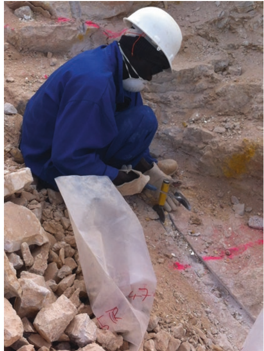
■ Fig. 4.7 Channel sample obtained with a hammer and chisel (Image courtesy of Martin Pittuck)
