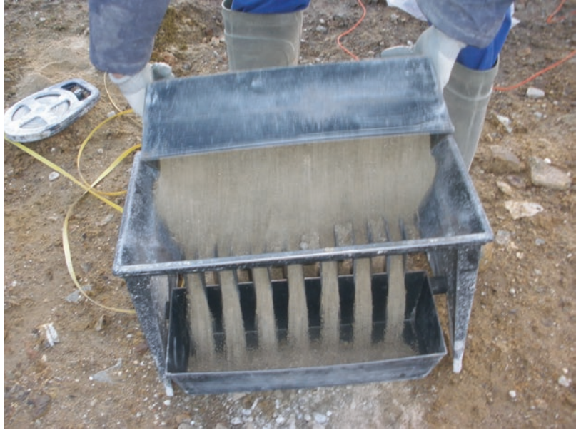
■ Fig. 4.17 Riffle division method (Image courtesy of Alicia Bermejo)
