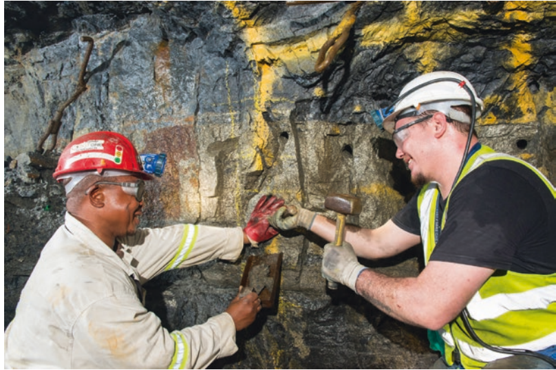
■ Fig. 4.8 Chip sampling (Image courtesy of Gold One Group Limited)
