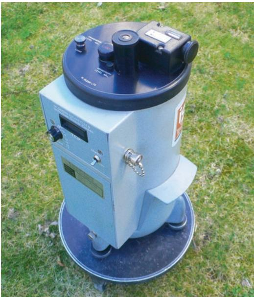
▣ Fig. 3.18 Gravimeter (Image courtesy of International Geophysical Technology)
