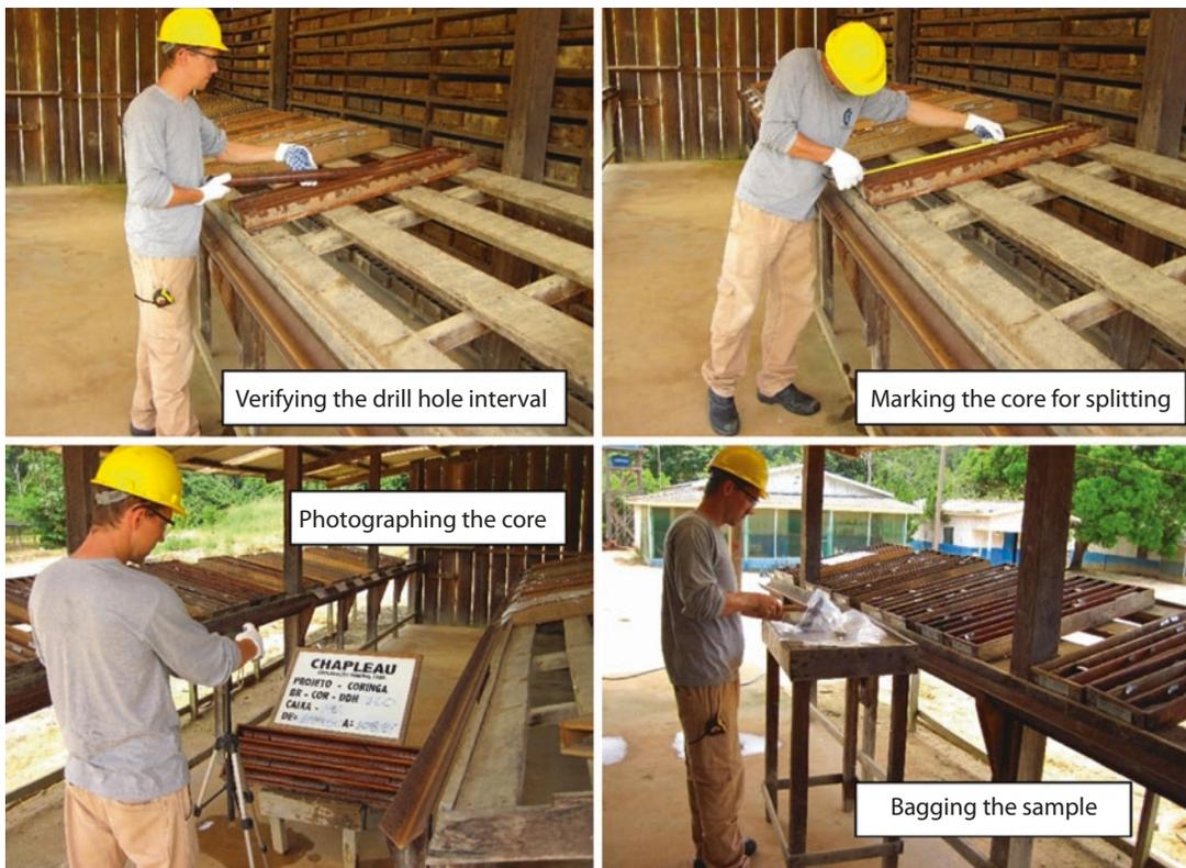
Fig. 3.75 Sampling procedure (Images courtesy of Anfield Gold Corp.)
