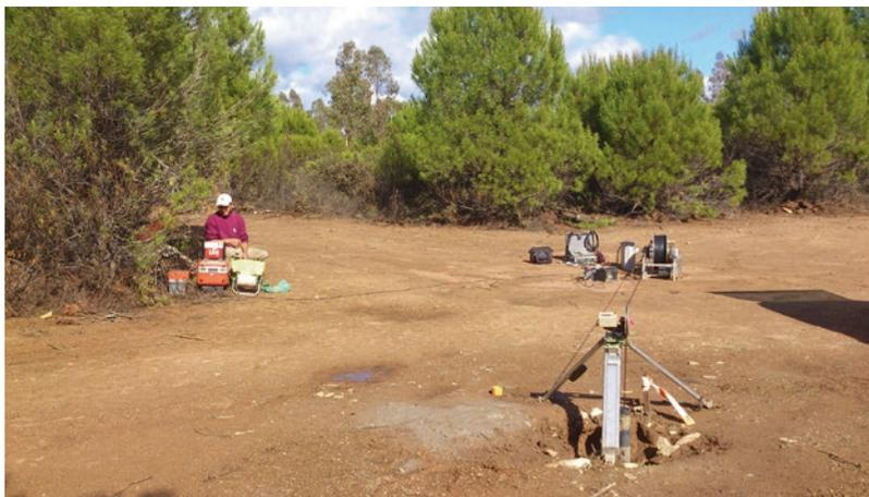
conductivity of layers down to 300 m below surface. Unlike conventional resistivity techniques, EM works without a physical contact to the ground, without electrodes, which is in advantage for use above ice, water, swamps, frozen, or arid ground.
