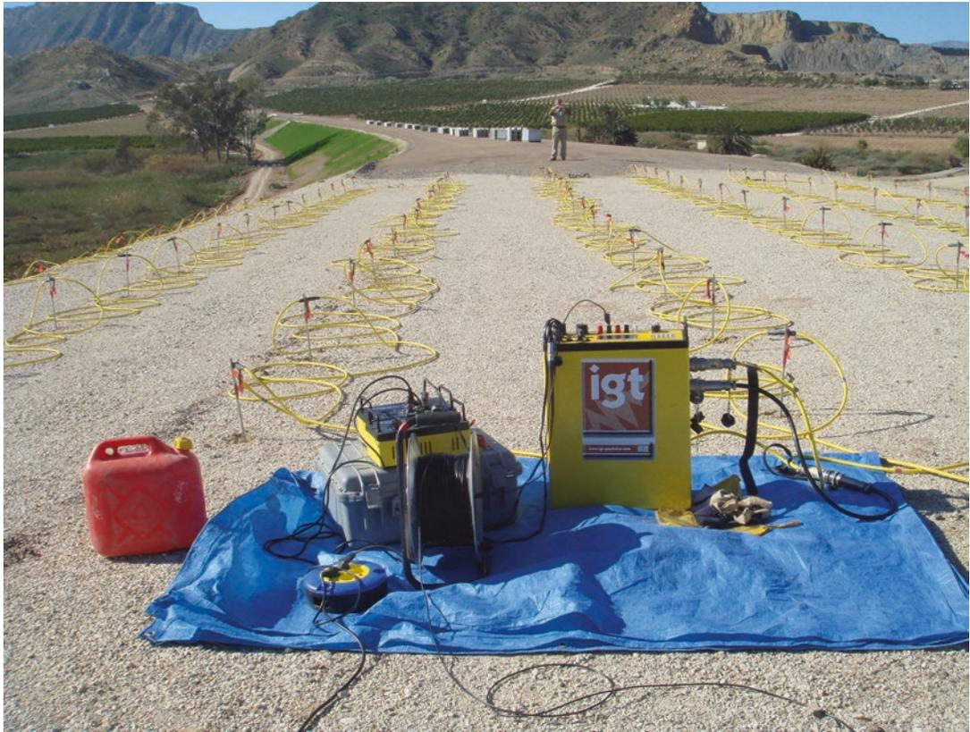
■ Fig. 3.22 Electrodes arrangement (Image courtesy of International Geophysical Technology)
