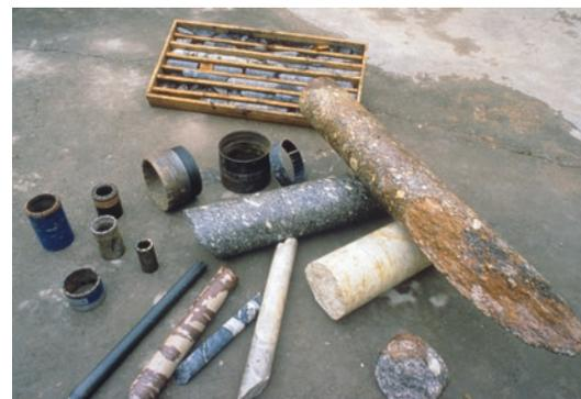
■ Fig. 3.54 Different core diameter sizes
