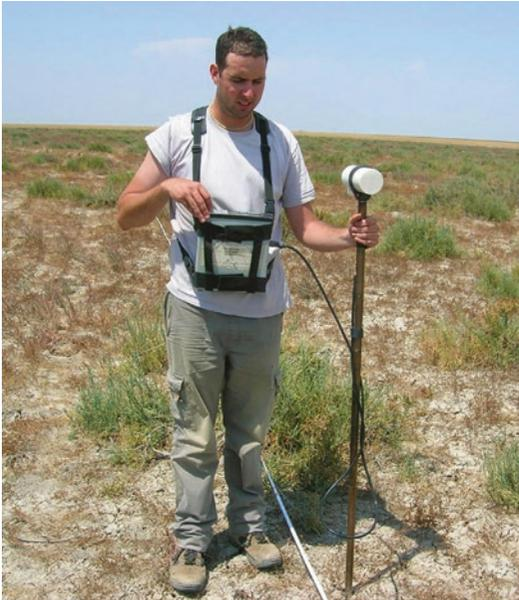
■ **Fig. 3.20** Magnetic survey (Image courtesy of International Geophysical Technology)
