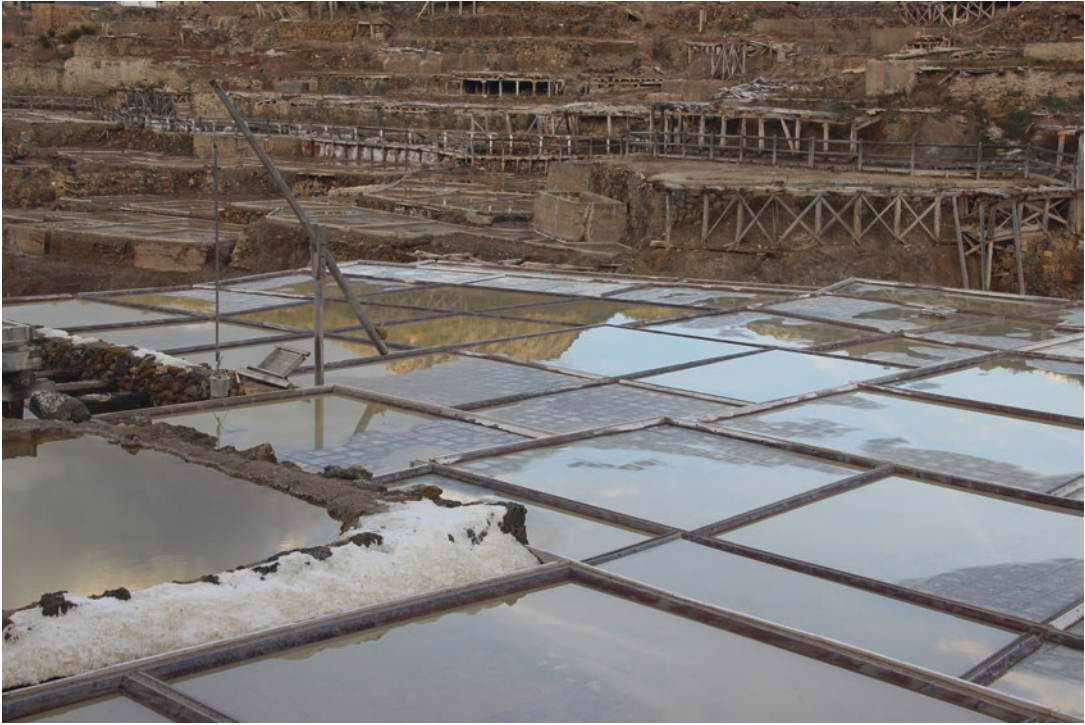
■ Fig. 2.50 Evaporation of brines to obtain common salt (Spain) (Image courtesy of José Pedro Calvo)
