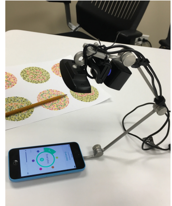
Fig. 2. iPhone with camera mounted to record and observe user interaction with the phone screen.
