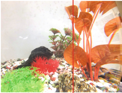
(b) The observer's view when water is filled with, in which the objects are skewed towards the right compared to (a).
