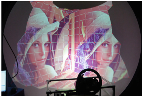
Fig. 7. Result of distortion correction in environment 1 (captured approximately 2 m behind the ideal viewpoint)
