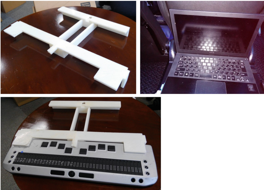
Fig. 3. The mobile braille display frame: assembled and in use
