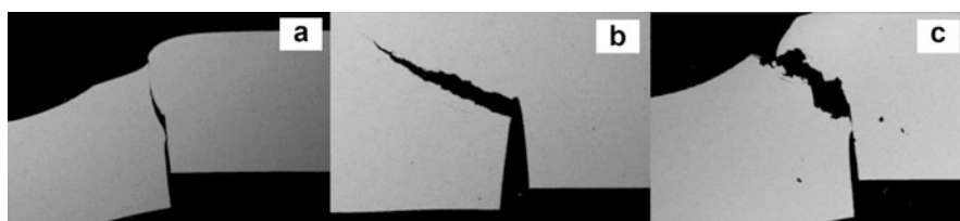
Fig. 3 Three different crack patterns observed at different temperatures (a): ductile fracture at 22°C, (b) brittle fracture at -196°C, (c) temperature-dependent transition fracture pattern
