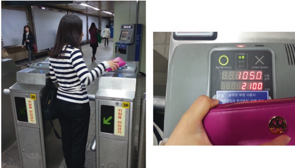
Fig. 12.5 The credit-based transportation card displays the fare and accumulated charges for the current month at the ticket gate (Photos by J. K. Lee)
