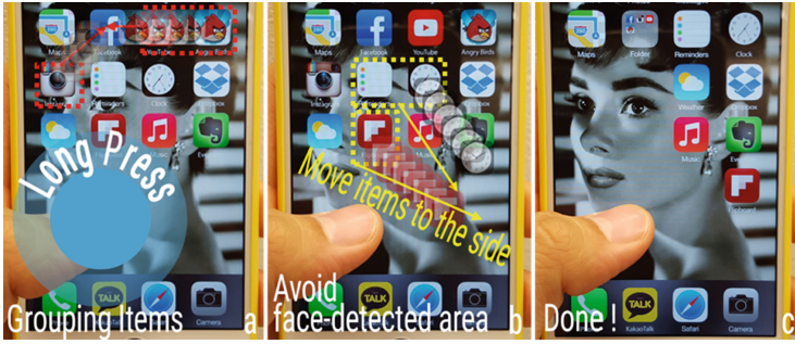
Fig. 6. Method of arranging icons on the proposing UI, (a) long press gesture triggers home screen items to be grouped, (b) items are moved to the side, (c) apps are rearranged
