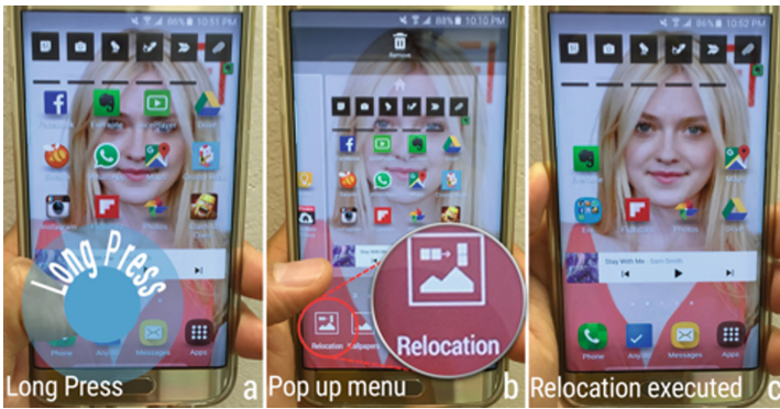
Fig. 7. Home screen prototype for Android OS, (a) long press gesture triggers the home screen setting menu, (b) menu is popped up with ‘Relocation’ button, (c) icons are rearranged
