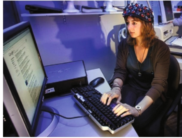
Fig. 1. The Hitachi 52-channel fNIRS device recording cognitive data while a participant completes a task.
