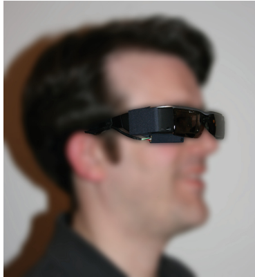
Fig. 1. Example of the eye-tracking enabled smart glasses with augmented reality capabilities based on the Epson Moverio BT-200.
