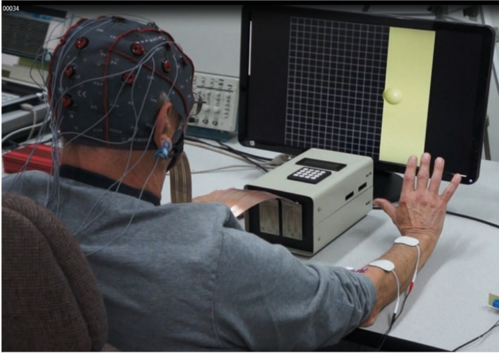
Fig. 2. BCI-EEG interventional therapy setup [8]
