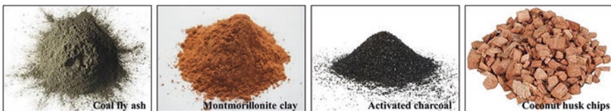
Fig. 3.3 Reactive media used in permeable reactive barrier for heavy metal removal from groundwater. Inorganic media, such as coal fly ash and montmorillonite clay, as well as organic media such as activated charcoal and coconut husk chips are often employed
