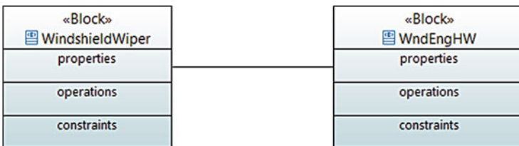
Fig. 2.6 An example principle—bidirectional coupling between two blocks
