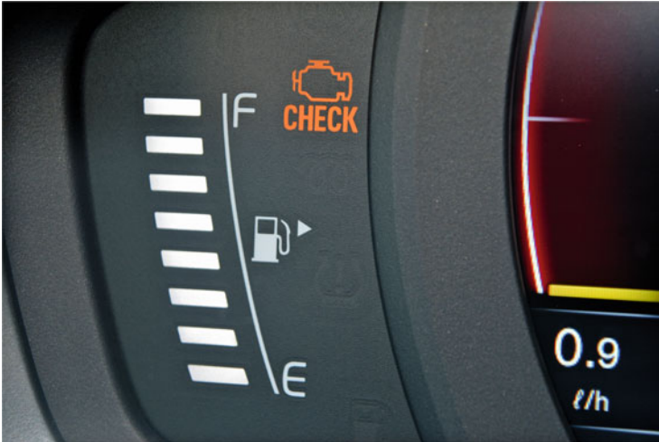
Fig. 6.3 Engine check control light indicating reduced performance of the powertrain, Volvo XC70
