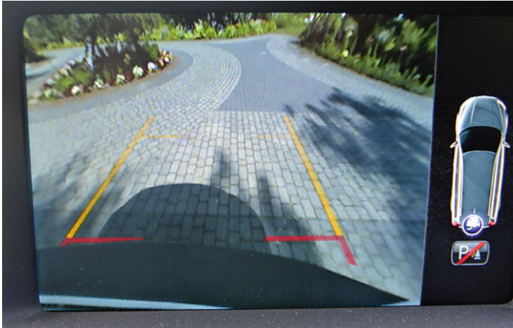
Fig. 6.4 Parking assistance camera showing the view behind the car while backing up, Volvo XC70
