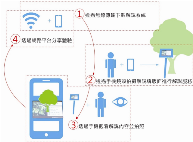
Fig. 3. Four steps to operate the prototype
