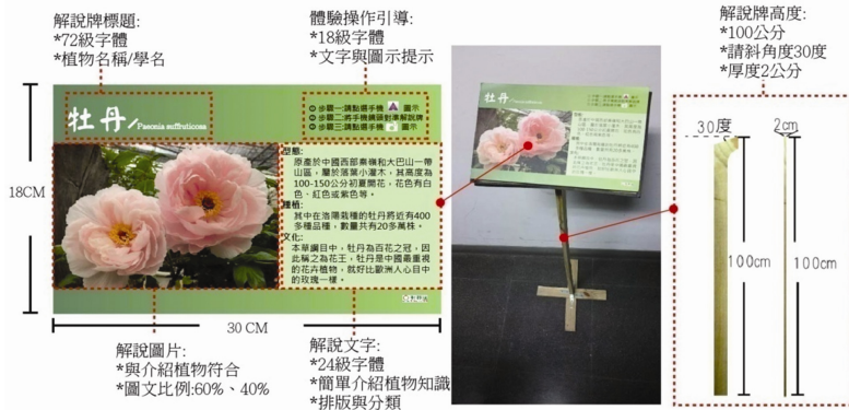
Fig. 6. Description hardware form
