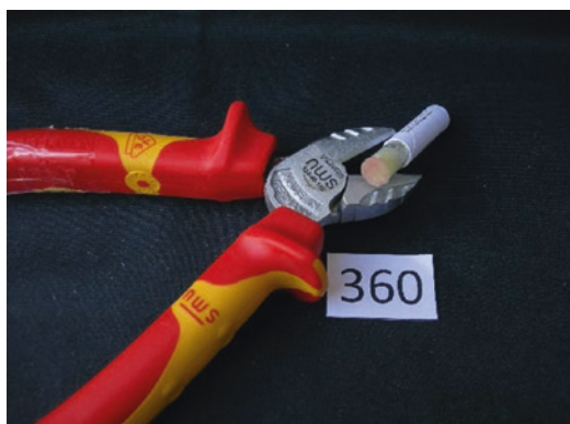
Fig. 14.1 Cobalt release from tools is rare: a positive spot test from the functional part of a pair of pliers
