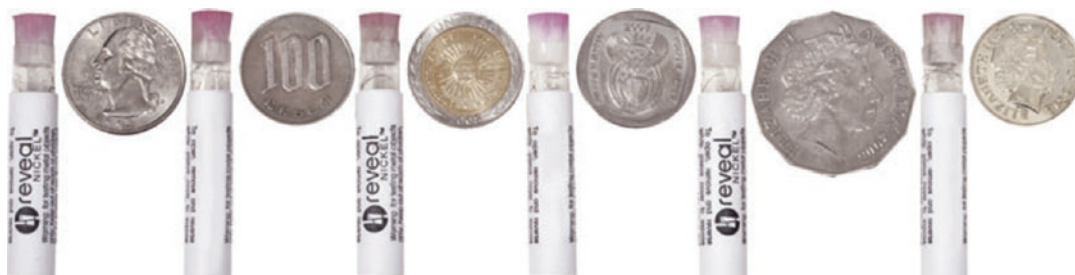
Fig. 16.1 Coins tested with the dimethylglyoxime test from the six major geographical regions according to the United Nations: a 0.25 US dollar coin (a quarter), a 100 Japanese yen coin, a 1 Argentinian dollar coin, a 2 South
