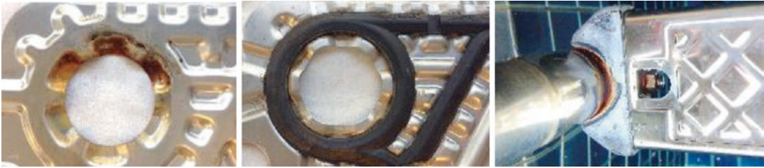
Fig. 2.2 The pictures to the left show crevice corrosion under a gasket in a stainless steel heat exchanger, and to the right , a stainless steel railing for a staircase leading into
