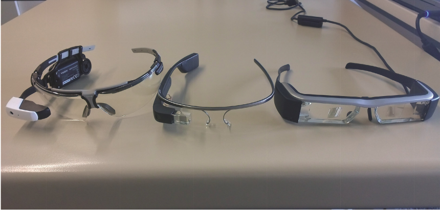
Fig. 1. Set of used smart glasses – Vuzix M100, Google Glass, Epson Moverio BT200
