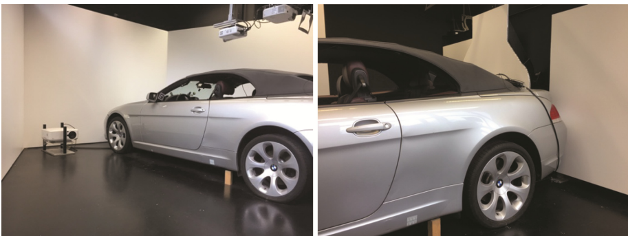
Fig. 2. Setup of the static driving simulator of the Institute of Ergonomics, TUM
