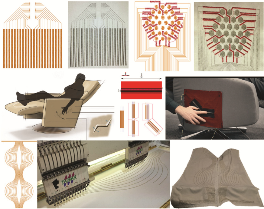
Fig. 5. Different stitch patterns for the three realized demonstrators (top: jacket, middle: armchair, bottom: curtain).
