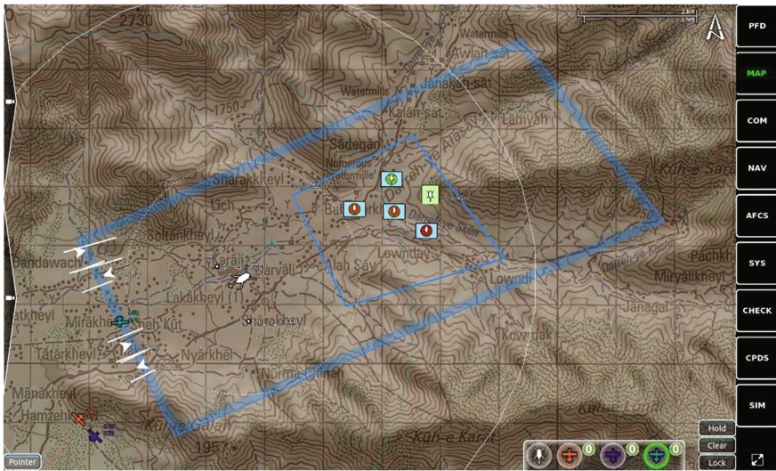
Fig. 8. Tactical map visualization of the landing point evaluation results displayed in the multi-function-display of our H/C simulator. The landing point quality is depicted color-coded in an easy-to-understand traffic-light representation.
