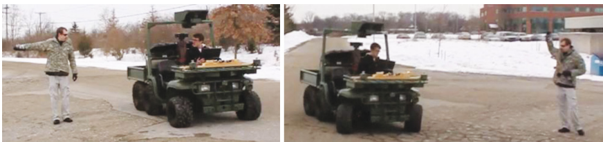
Fig. 3. Examples of gestures being given to control a large UGV (person on board the vehicle is a safety operator.)
