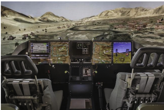
Fig. 9. IFS helicopter simulator cockpit
