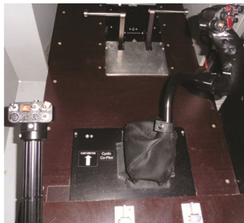
Fig. 7. Flight controls of the helicopter simulator: collective, cyclic and pedals.
