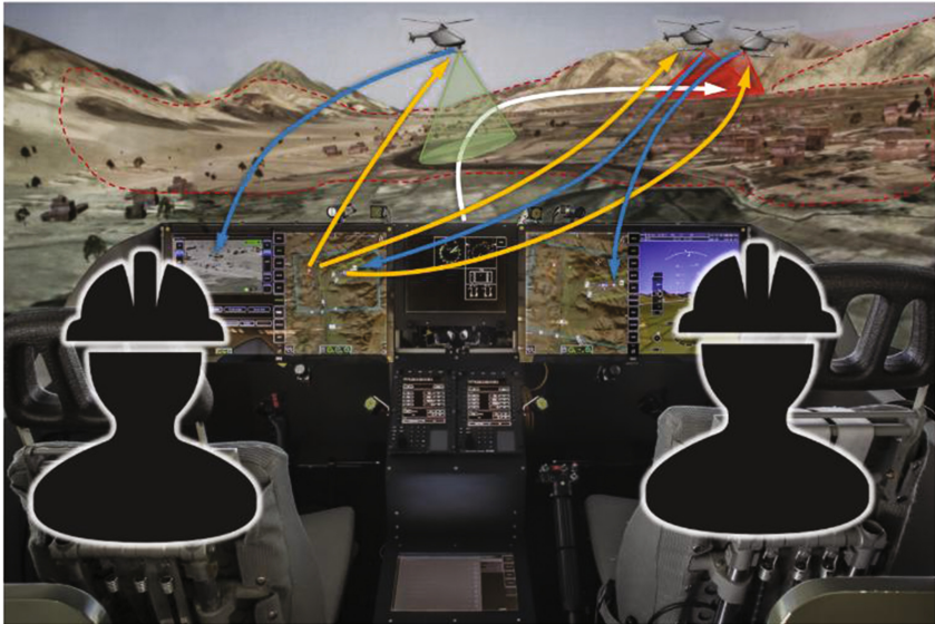
Fig. 1. MUM-T principle in our H/C mission simulator at the IFS. The PiC (left) is commanding multiple UAVs to reconnoiter its flying route (white) and mission-critical areas, i.e. the desired landing zone in the background (red). (Color figure online)
