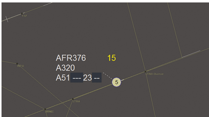
Fig. 4. Advisory countdown (yellow) shown at the controller radar display (Color figure online)
