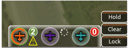
Fig. 6. UAV Dock. Left UAV has two tasks and warnings, center UAV is planning, and right UAV is offline. (Color figure online)
