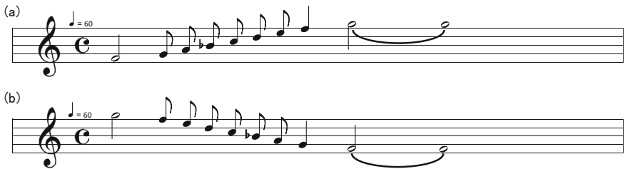
Fig. 4. Sounds presented during acceleration and deceleration. Upper (a): musical score indicating the sound presented during acceleration. Lower (b): musical score indicating the sound presented during deceleration. Both sound patterns lasted 6 s.
