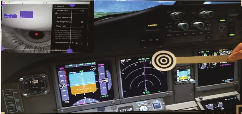
Fig. 4. Eye camera adjustment view and manual calibration process
