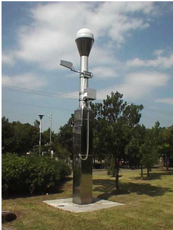
Fig. 5.12 A GEONET GNSS-based CORS station in Japan. Source Geospatial Information Authority of Japan
