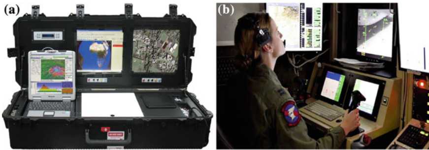
Fig. 20.4 a An example of transportable UAV ground control station; b An example of large Ground Control Station (GCS), the MQ-9 Reaper UAV GCS
