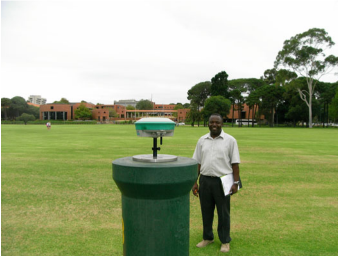
Fig. 5.5 Reference station, pillar 18 at Curtin University, Bentley Campus, Australia
