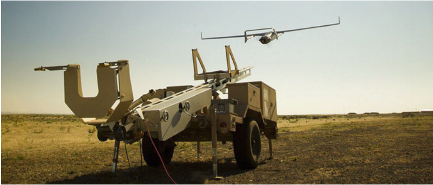
Fig. 20.5 An example of large UAV launcher
