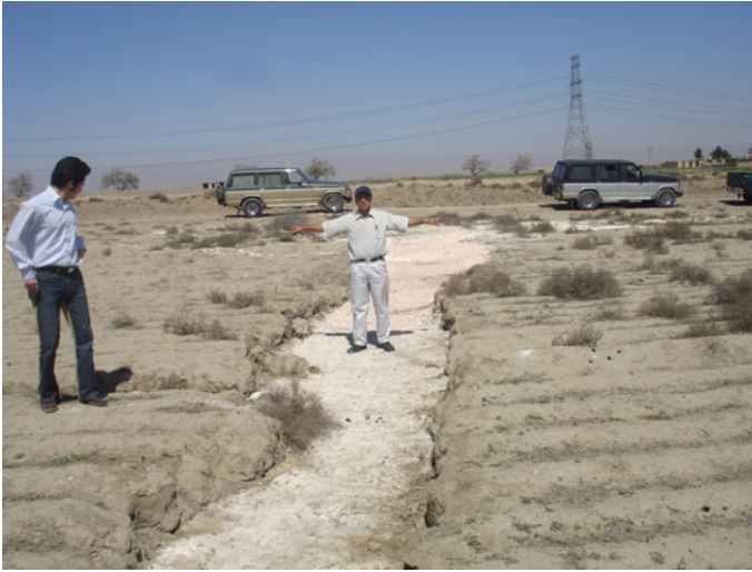
Fig. 17.5 An example of surface fissures in Mashhad Valley caused probably by excessive groundwater withdrawal and associated aquifer-system compaction. The fissure is located northwest of Mashhad City and to the east of the Tous. A GNSS station is marked by a triangle in Fig. 17.4 near the city of Tous. Source Motagh et al. [41]
