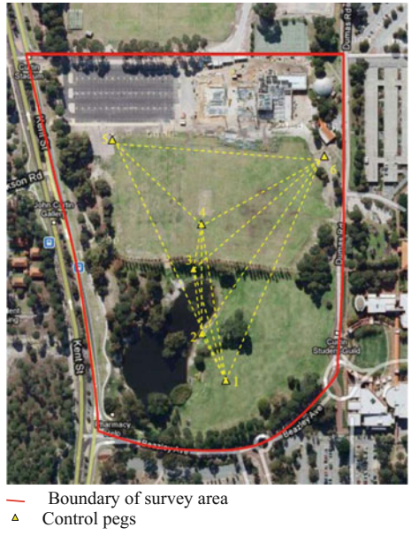
Fig. 8.1 Edinburgh Oval, Curtin University’s study area with control peg network. Source http://maps.google.com/maps
