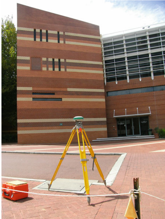
Fig. 4.3 A static receiver stationed on a tripod at point G2 of Curtin University (Bentley Campus), Australia
