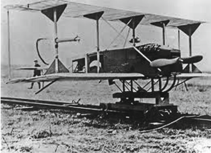
Fig. 20.1 Hewitt-Sperry Automatic Airplane, prototype of today's cruise missiles. The first demonstration of the model of UAV, was created and passed the flight test in 1917
