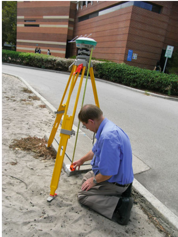
Fig. 5.6 Setting up a GNSS antenna and measuring its height at Station John Walker (JW) at Curtin University, Bentley Campus, Australia
