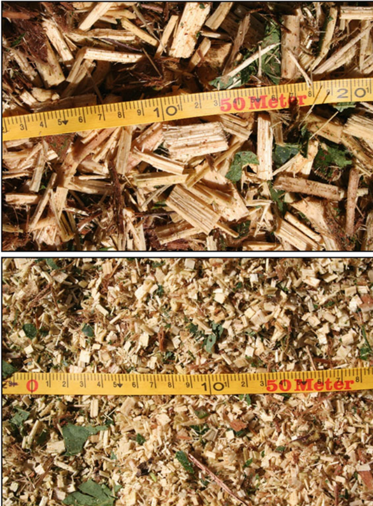
Fig. 3 Woodchips length: 30 mm ( top ) and 5 mm ( bottom )
