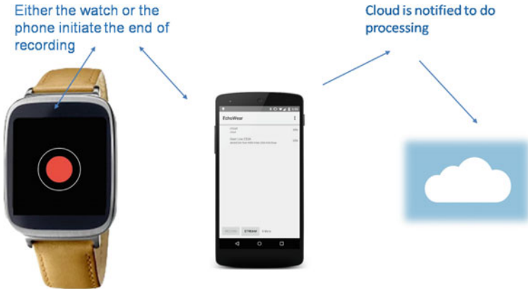
Fig. 3 The flow of information and control between three main components of the medical IoT system for smartwatch-based speech treatment [12]. The smartwatch is triggered by the patients with Parkinson’s disease. At fixed timings set by patients, caregivers or their speech-language pathologist (SLPs), the tablet triggers the recording of speech data. The smartwatch interacts with the tablet via Bluetooth. Once tablet gets the data from smartwatch, it send to the Fog devices that process the clinical speech. Finally, the features were sent to the cloud from where those could be queried by clinicians for long-term comparative study. SLPs use the final features for designing customized speech exercises and treatment regime in accordance with patient’s communications deficits
