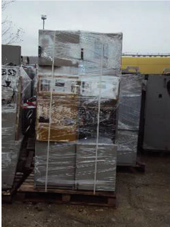
Fig. 1 Correct strapping of equipment to wooden pallets
