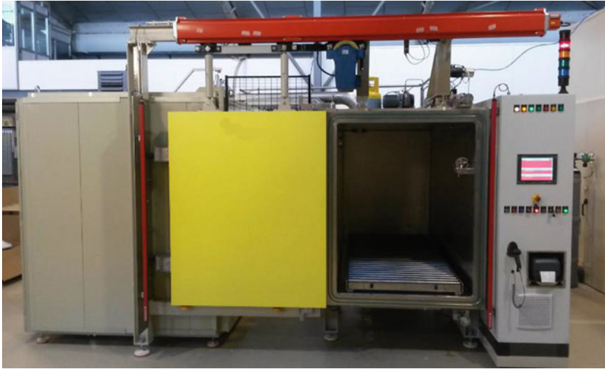
Fig. 3 A cabinet used for gas filling and recovery for MV equipment
